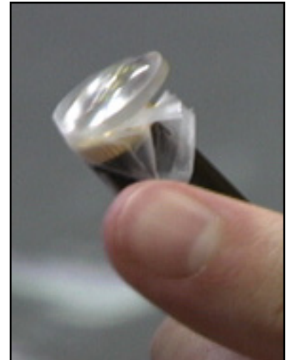
Tape lens onto laser pen.
