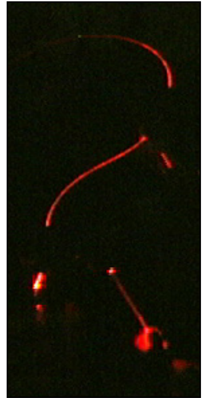
Laser beam shining through flexible tubing.
