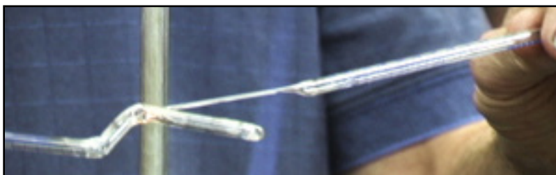
Stretching the second tube to make an "ear."
