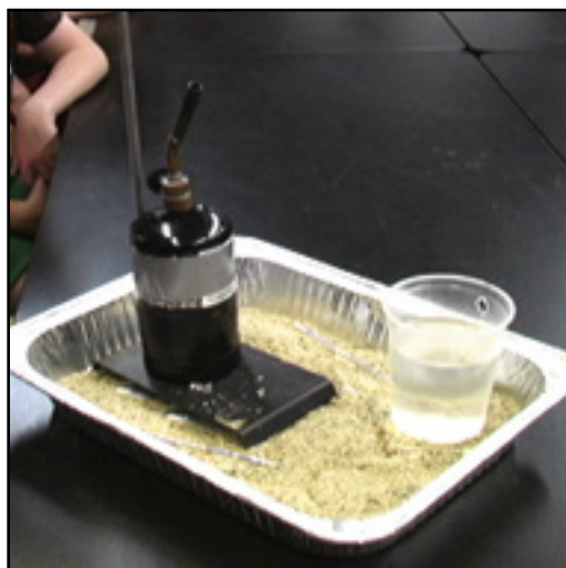
Propane torch duct-taped to lab stand, with sand and water in aluminum pan.
