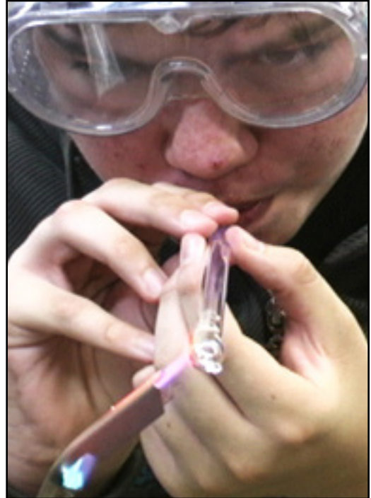
Blowing a bubble in the glass tube.
