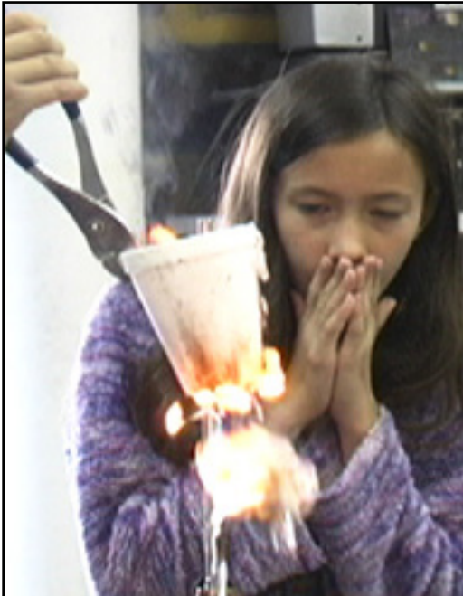
The bottom falls out of this styrofoam cup as it quickly burns.
