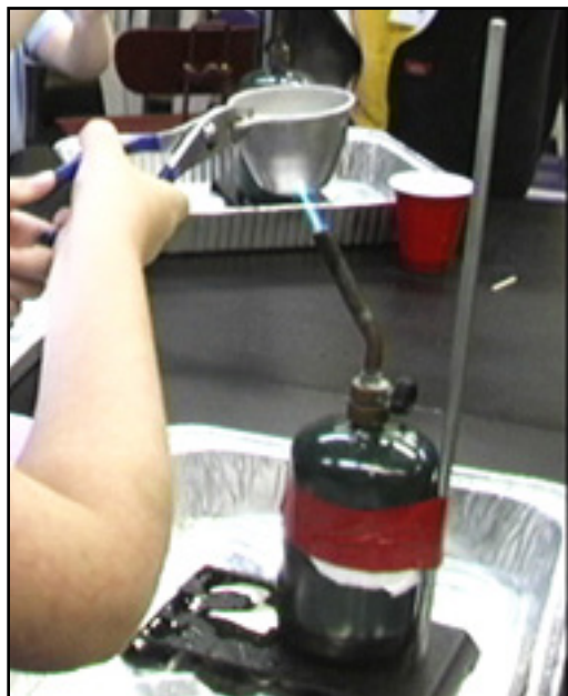
Torch secured to vertical rod with duct tape.
