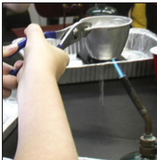
Holding aluminum cup with pliers over flame.
