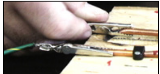
Connecting boards with alligator clips.
