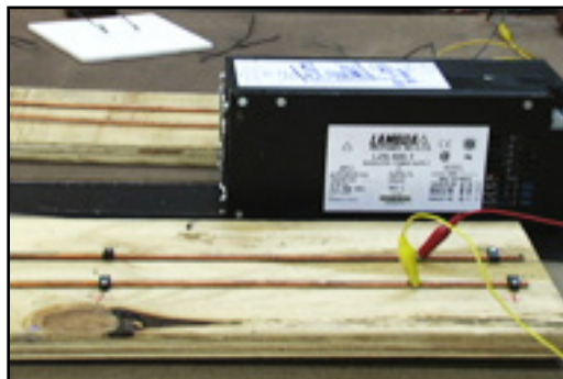
Power Supply with Wires mounted on Board
