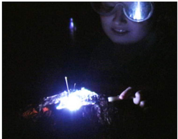
At Left and Above: Shorting out the capacitor with foil.
