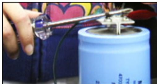
Using screwdriver to short out capacitor.
