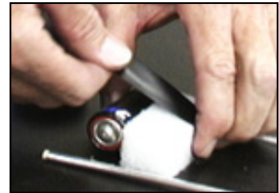
Tape one end of the battery to one chopstick, then tape the foam block to the battery.
