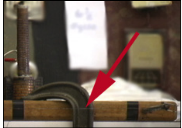
A thin wire is stretched between electrical connectors
