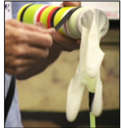
Stretch the opening of the glove over the end of the tube and secure with electrical tape.
