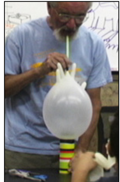
Place end of tube against table and blow into straw to check for an airtight seal around the Tube.
