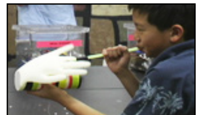
To make the glove-o-phone work, turn the tube so that the closed end is pointing away from you and the glove is stretched taut over the opening.
