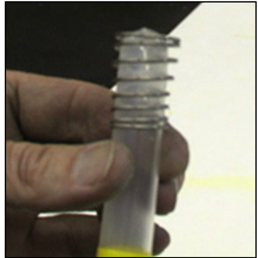
Test tube with a spring on the bottom. This holds the other test tube straight until the glue dries.
