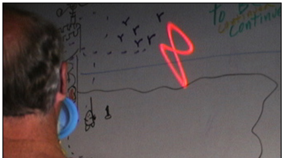
When you shout into the hole in the cup, the laser makes an image on the wall.
