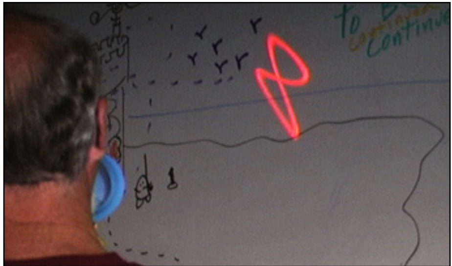
When you shout into the hole in the cup, the laser makes an image on the wall.
