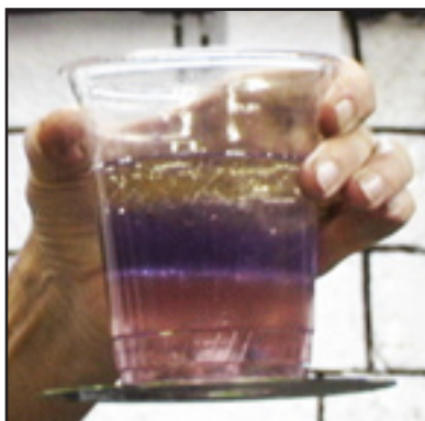
Top: soybean oil; Middle: brake fluid; Bottom: water
