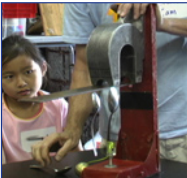
Stainless steel sticks to the magnet.
