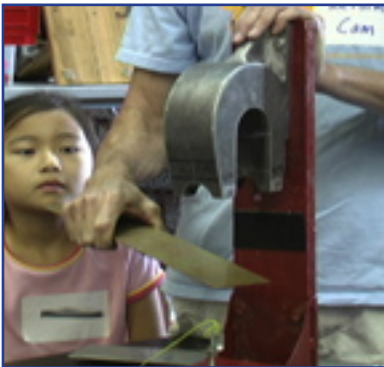
Brass doesn't stick to the magnet.
