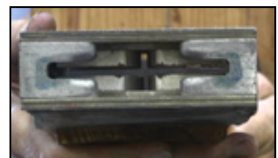
Magnets inside hard drive.
