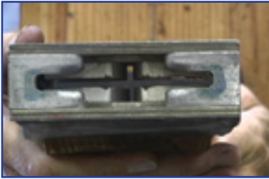
White magnets inside hard drive.
