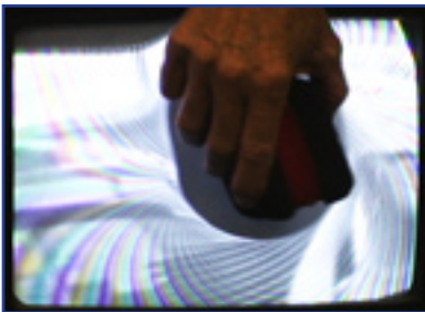
The magnet disrupts the tv image.
