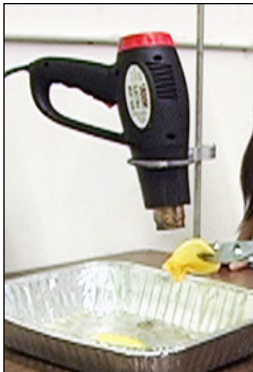
Hot air gun, lab stand, aluminum pan.
