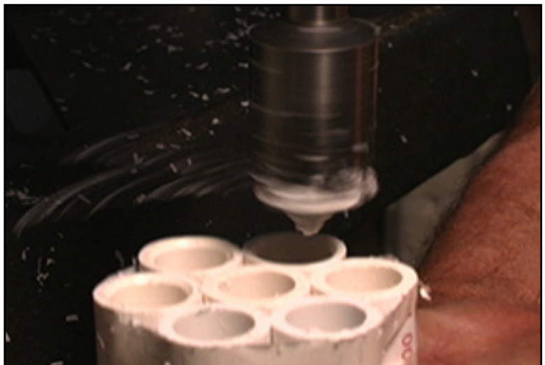
Bevel the edges with a countersink so they don't tear the balloons.
