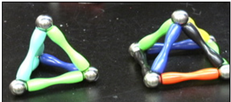
Triangle pyramid (at left) is stronger than a square-base pyramid.
