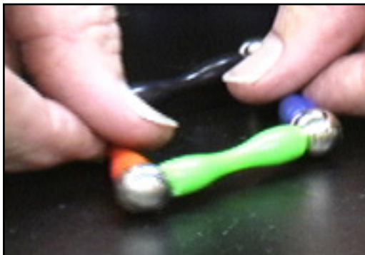
A square twists out of shape easily.
