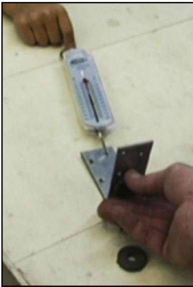
Pulling the magnet to make the angle bracket pull on the scale.
