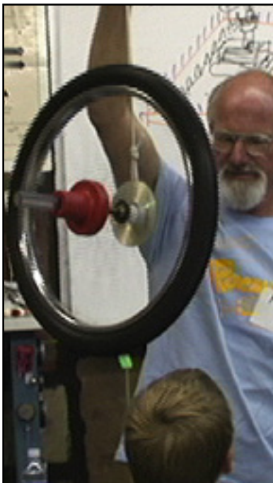
The spinning wheel, held only by a rope at one end of the handle, doesn't fall.
