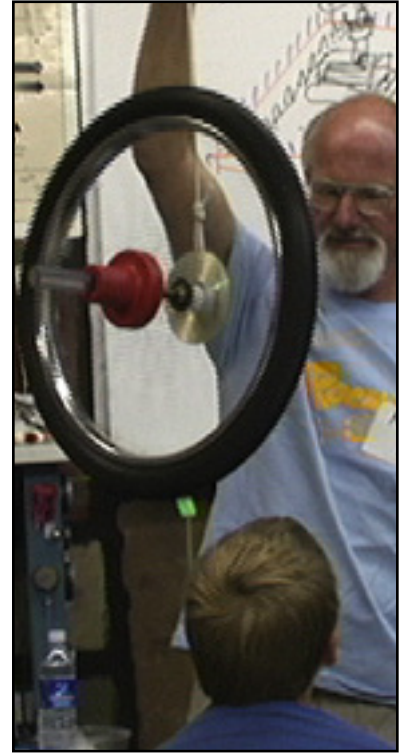
The spinning wheel, held only by a rope at one end of the handle, doesn't fall.
