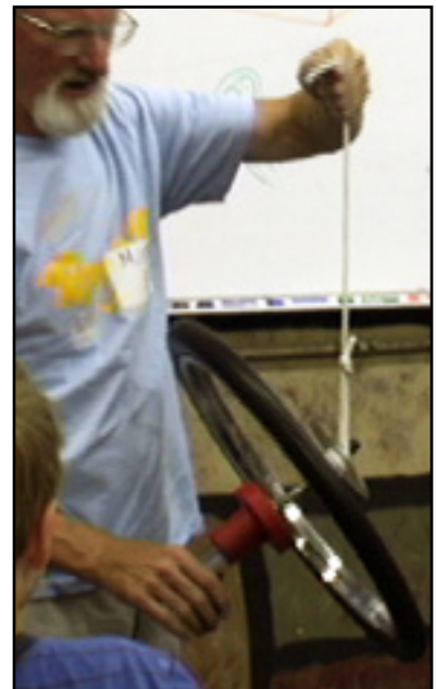
If you stop the rotation, the wheel starts to fall over.
