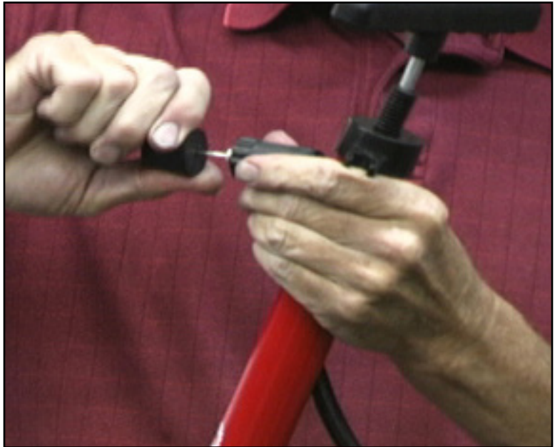
Insert the needle through the small hole in the rubber cork.
