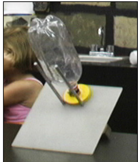
Bottle mounted on cork and launch pad set at an angle.
