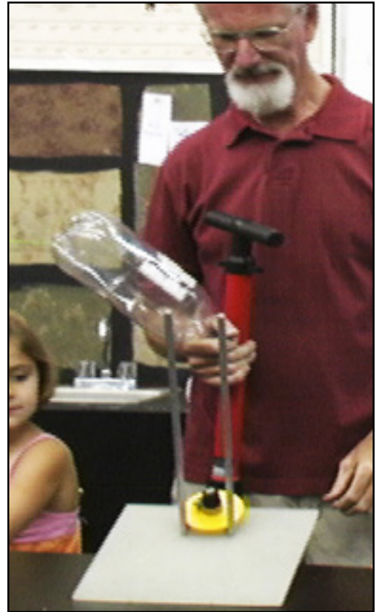
Bottle, bicycle pump, and launch pad with rubber cork in place.
