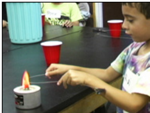
Heating bent wire with alcohol lamp.
