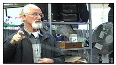
Instructor rotates the spring to make different wave lengths.
