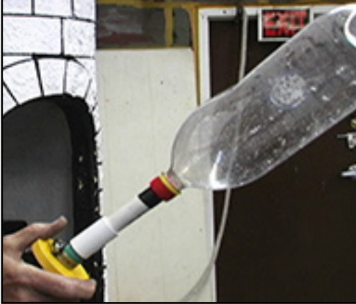
Cork from bicycle pump attached to pipe.
