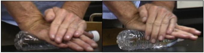
Bottle filled with Air (at left) squishes more than Bottle filled with Water (at right).
