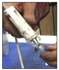
Gluing the Washers on
