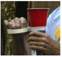
Attach the cup to the tube with masking tape.
