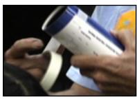
Wrap masking tape around the cardboard tube to hold it in place.
