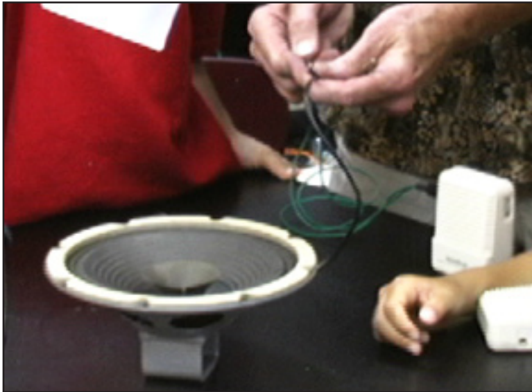
Hooking up the amplifier to a speaker with alligator clips.
