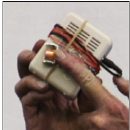
Amplifier with pickup coil.
