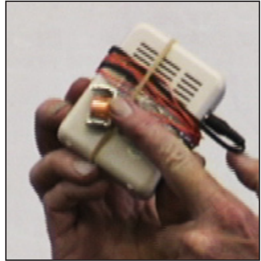
Amplifier with pickup coil.
