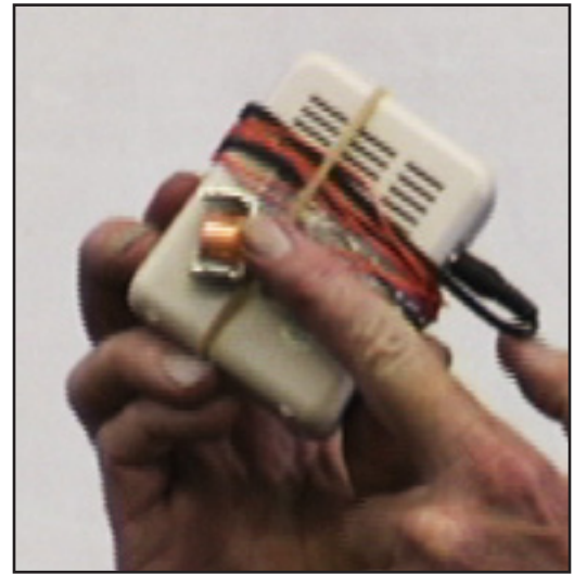
Amplifier with pickup coil.
