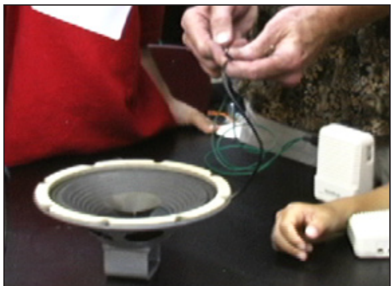
Connecting speaker to amplifier with alligator clips.
