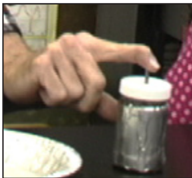
Safe way to check for charge.
