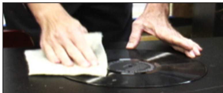
Rubbing vinyl record with wool to charge it up.
