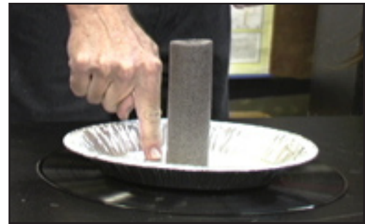
Place pie tin on charged record and touch it with fingertip to discharge a spot.
