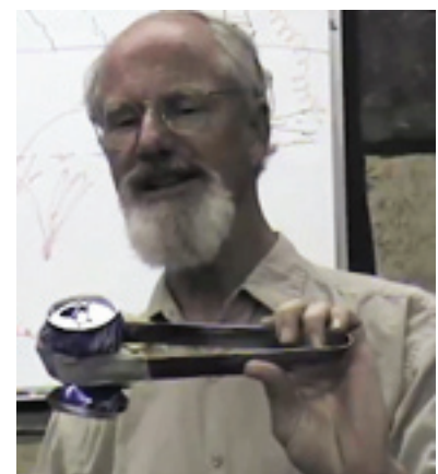
When water vapor turned back into water, it created a vacuum that crushed the can.
