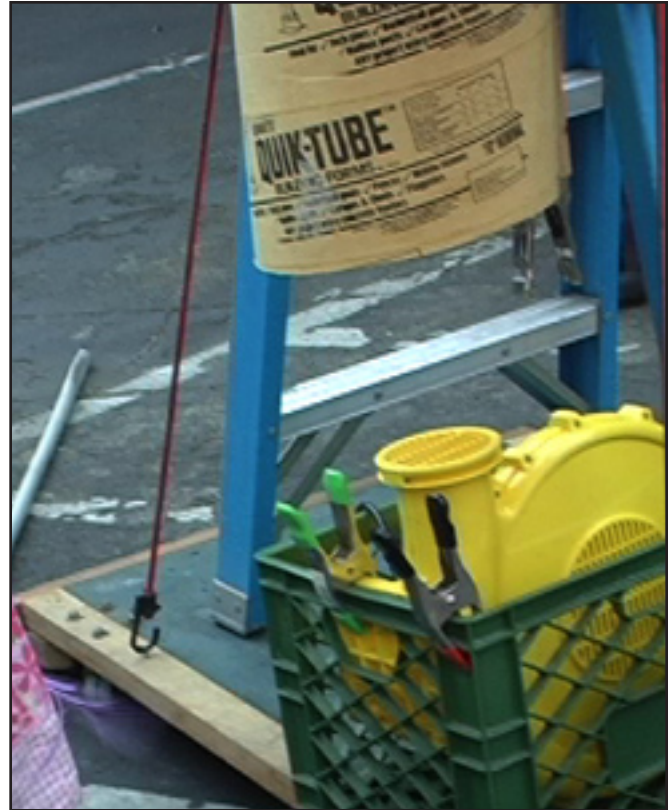
Bungee cords secure ladder to eye hooks in wheeled platform. Spring clamps secure fan to crate.
