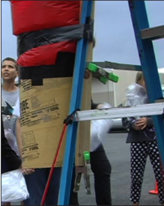
Bottom of balloon is taped to cardboard tube. Tube is clamped to 2"x4", which is clamped to ladder. More tape is wrapped around tube, 2"x4" and ladder. Bungee cords secure ladder to platform below.
