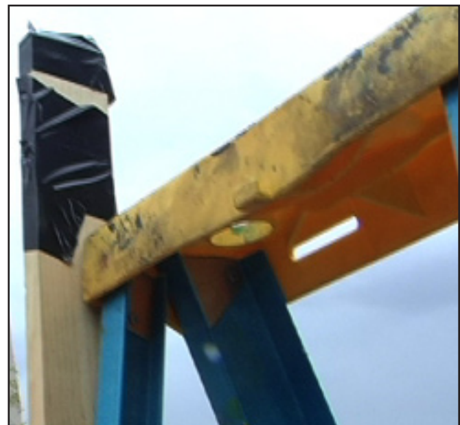
Tape covers top of 2" x 4" to keep rough edges from damaging balloon.
