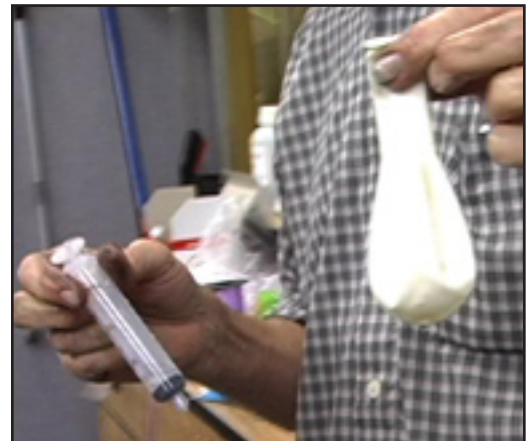
Syringe is used to inject 15 ml. of water into balloon.
