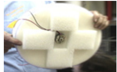
Motor mounted on underside of foam disk.
