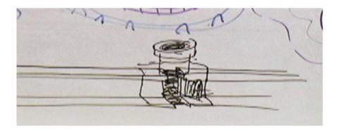
• Thermite was used to join railroad tracks. A mold was placed on each section of the track, then a pot of thermite was placed above the gap and burned. The molten iron filled in the mold, then filled in the gap between the tracks.
