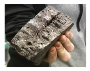
• Show a fragment of thermite left over from a track join, with iron oxide crystals in the middle.
