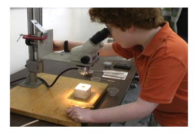
• Instructor sets up a firebrick under a microscope. Students place their magnets on it so they can view the iron bits.
